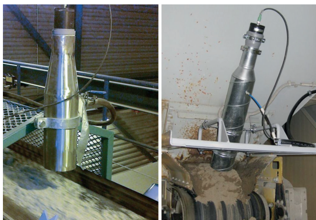
POLARMOIST installed over a conveyor belt on the left and on a silo feeder on the right to measure water content in aggregates.
