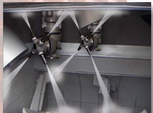
A80R heads installed in a twin-shaft mixer
