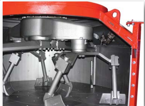
A80R head installed in access cover of planetary mixer
